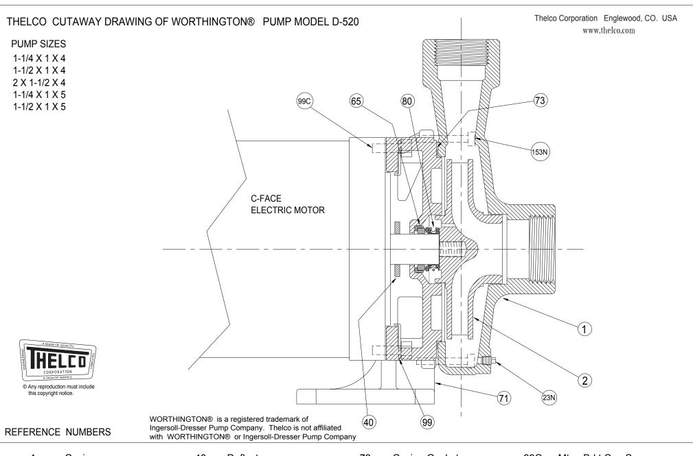
Casing Gasket 99C Mtng Brkt Cap Screw Casing Deflector 73 40 Impeller 65 Mechanical Seal Seat\* 80 Mechanical Seal Rotor\* 153N Casing Cap Screw 1/4" Pipe Plug 99 C-Washer 23N 71 **Mounting Bracket**
